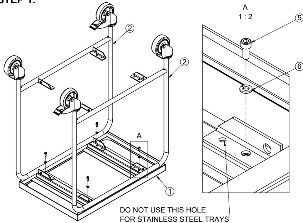
PUT ONE OF THE TRAYS UPSIDE DOWN ON A SOFT SURFACE AND PLACE THE FRAMES AS SHOWN IN THE PICTURE ABOVE. USE THE INCLUDED M6 HEX-KEY TO FASTEN THEM WITH SPRING WASHERS AND M6-SCREWS.
