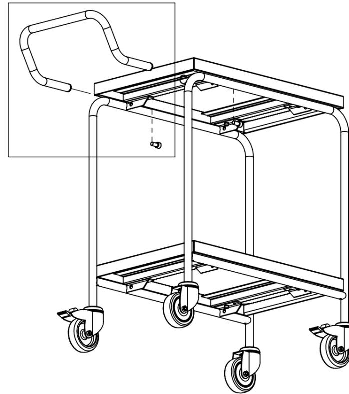
USE THE INCLUDED M10 HEX-KEY TO FASTEN THE HANDLE WITH M10-SCREWS.
